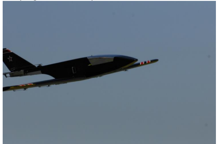
Chris Littles LDS JetMach powered by a Kingtech K-80 Turbine running on kerosene fuel.
